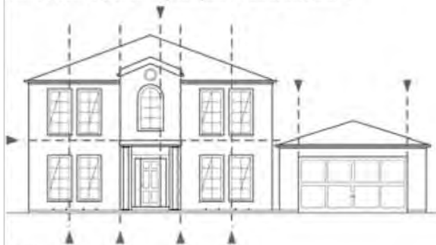
Unitex Base Board: Guide for Control / Expansion Joints - Front Elevation (use same principles for other elevations)
